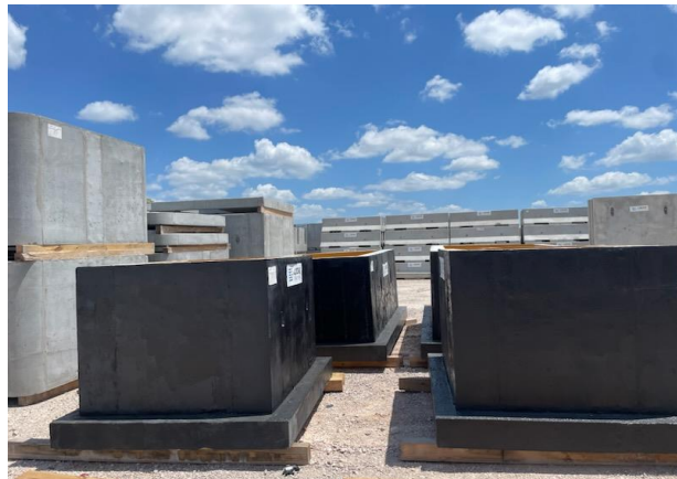
Fig. C (2-Years later) No blistering or delamination on impact zones
